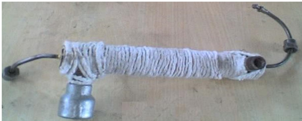
Figure 3.8: Heat exchanger with thermal insulation
