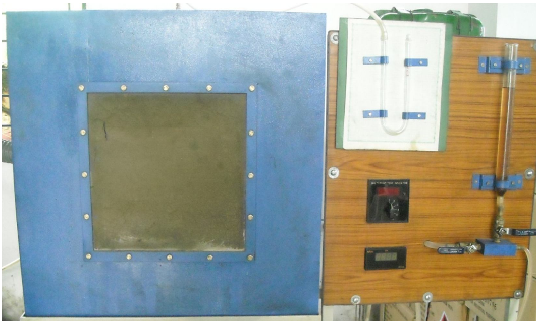
Figure 3.16: Apparatus to measure the rate of fuel and air consumption
