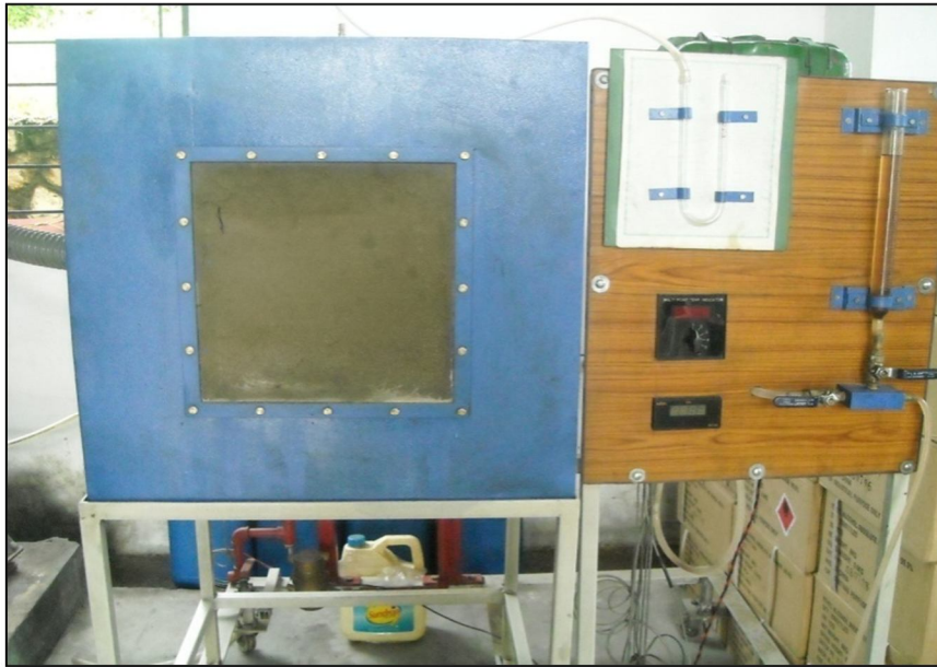
Figure 3.6 : Apparatus to measure rate of fuel and air consumption
