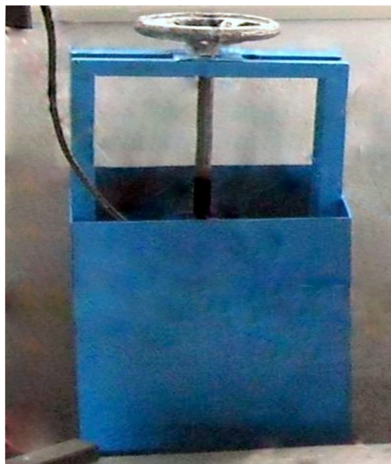
Figure 3.4 : Engine loading system
