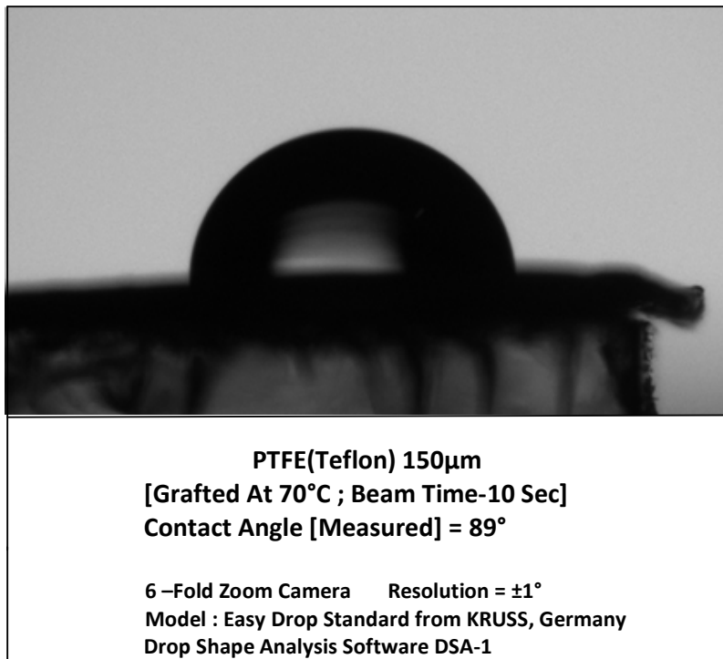
Fig. 7.8 (d) : DSA-1 Output of treated PTFE (10 sec) with grafting temperature 70°C (Contact Angle = 89°)
