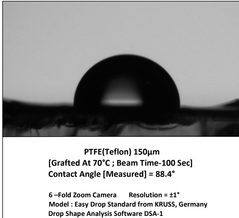
Fig. 7.9 (d) : DSA-1 Output of treated PTFE (100 sec) with grafting temperature 70°C (Contact Angle = 88.4°)
