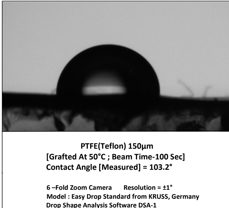
Fig. 7.9 (b) : DSA-1 Output of treated PTFE (100 sec) with grafting temperature 50°C (Contact Angle = 103.2°)
