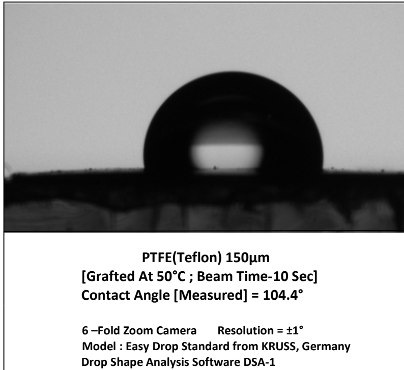
Fig. 7.8 (b) : DSA-1 Output of treated PTFE (10 sec) with grafting temperature 50°C (Contact Angle = 104.4°)
