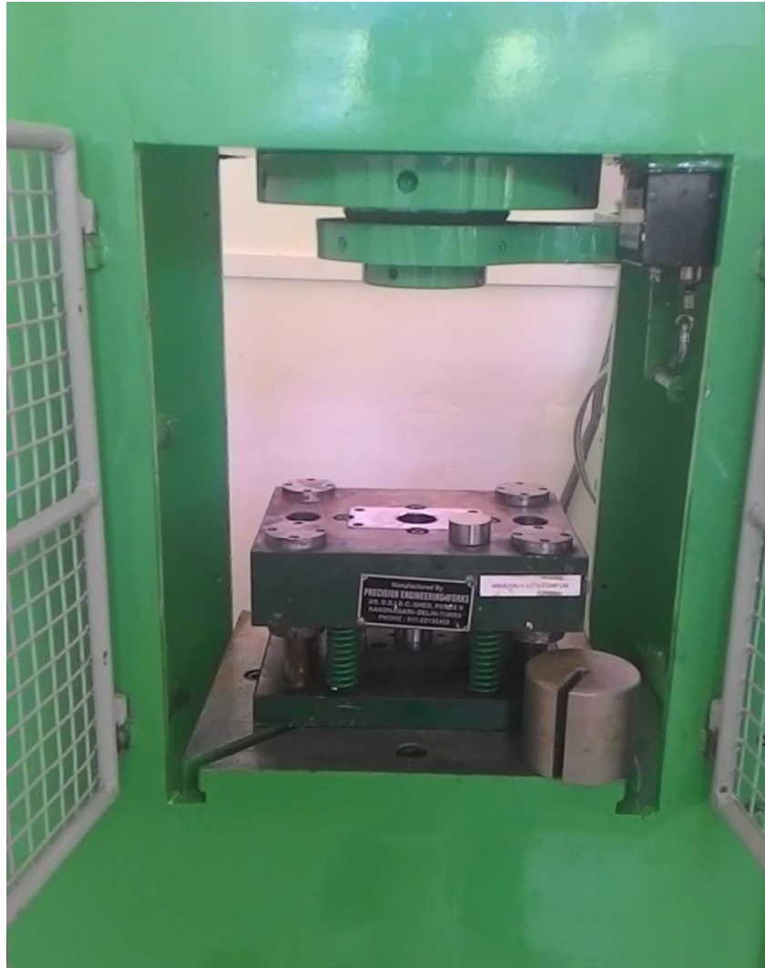
Figure 3.4: Hydraulic Pressing Machine used for Cold Compaction
