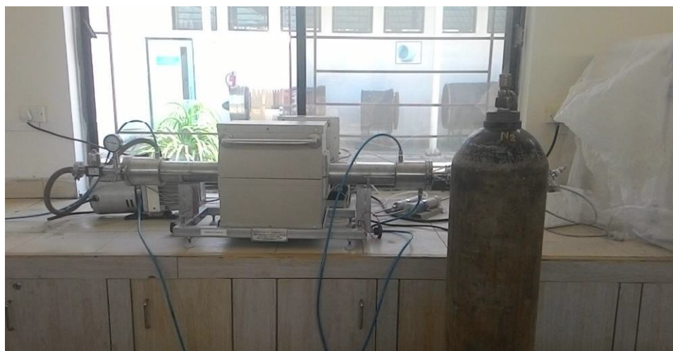
Figure 3.8: Tubular Furnace for Sintering process
