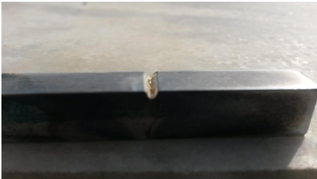
Appendix Figure1. 4 Bare Material Impact Test Specimen
