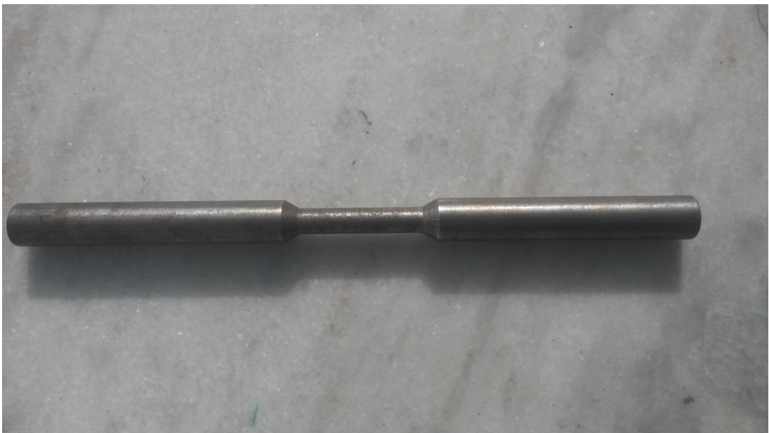
appendix figure1. 3 Bare Material Tensile Test Specimen
