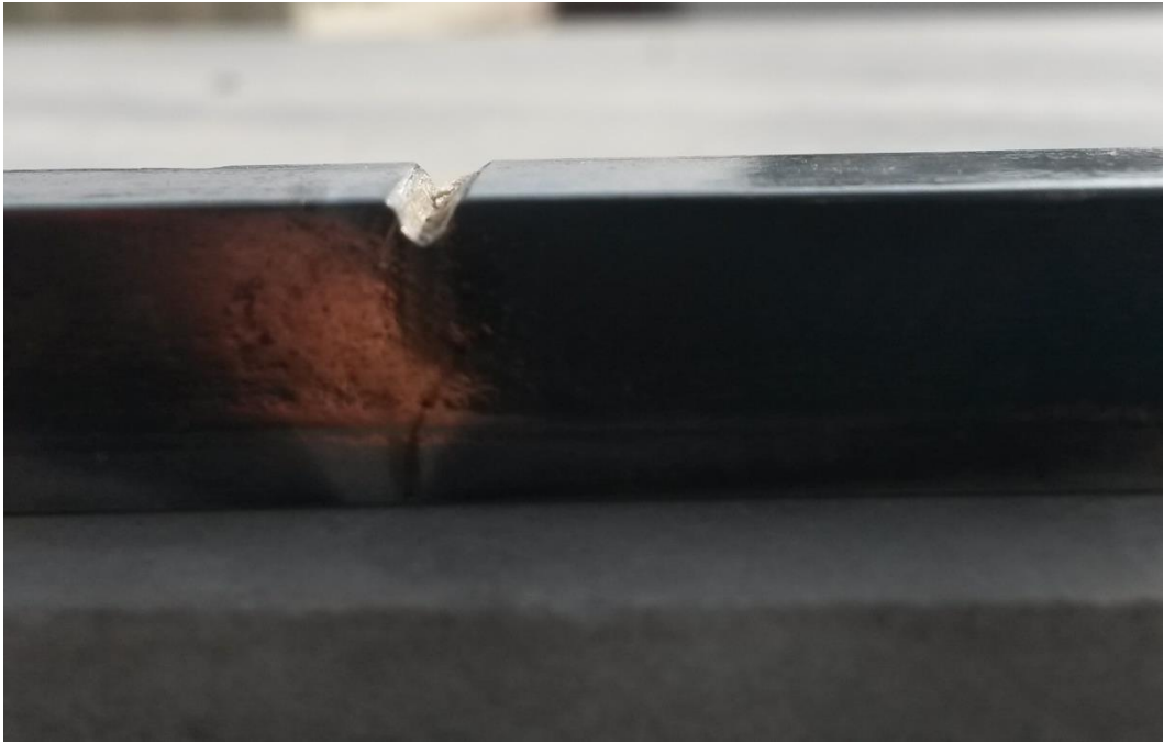
Appendix figure1. 5 Cu-Ni-Cr Coated Material Impact Test Specimen
