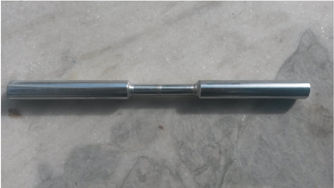
Appendix figure1. 2 Cu-Ni-Cr Coated Tensile Test Specimen
