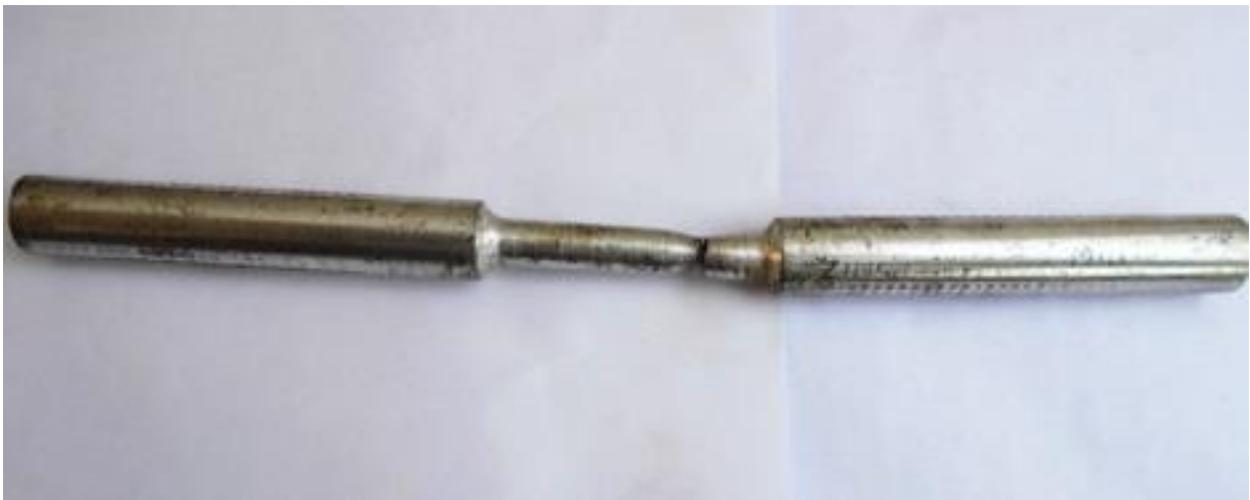
Fig 17: Zinc Coated Corroded UTM Test Specimen
