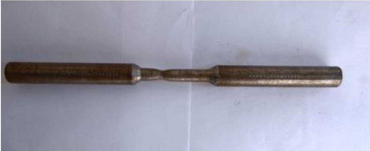
Fig 14: Bare UTM Test Specimen
