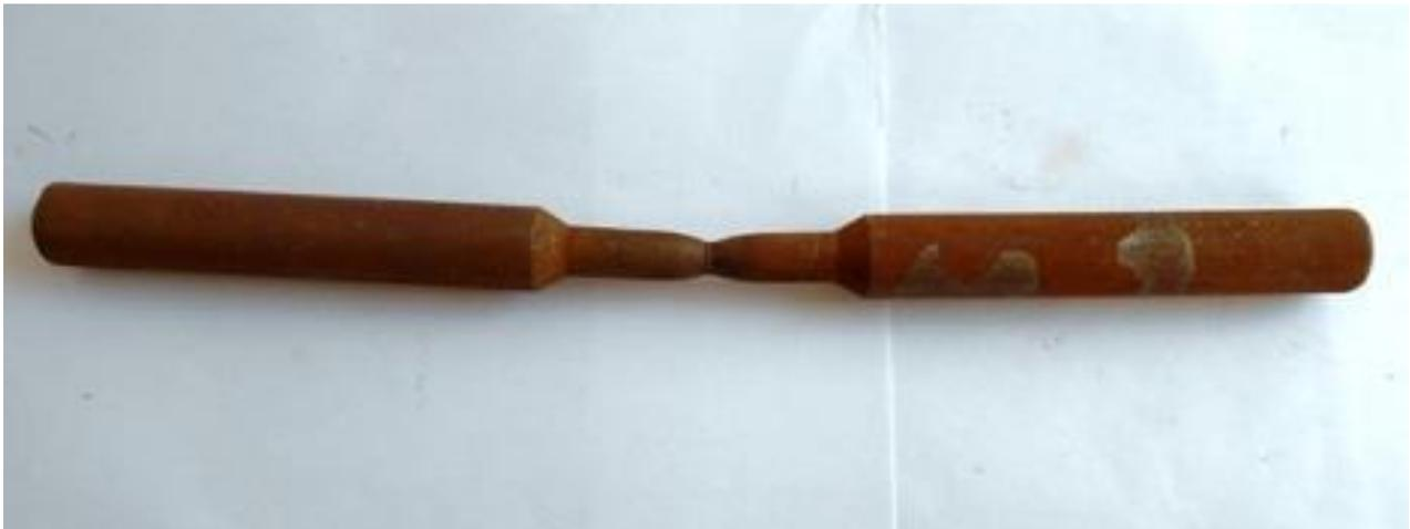
Fig 15: Bare Corroded UTM Test Specimen
