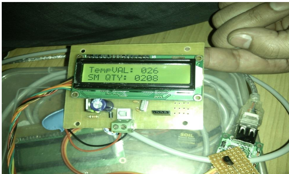
Fig.6.7 Sensor node with temperature sensor and soil moisture sensor
