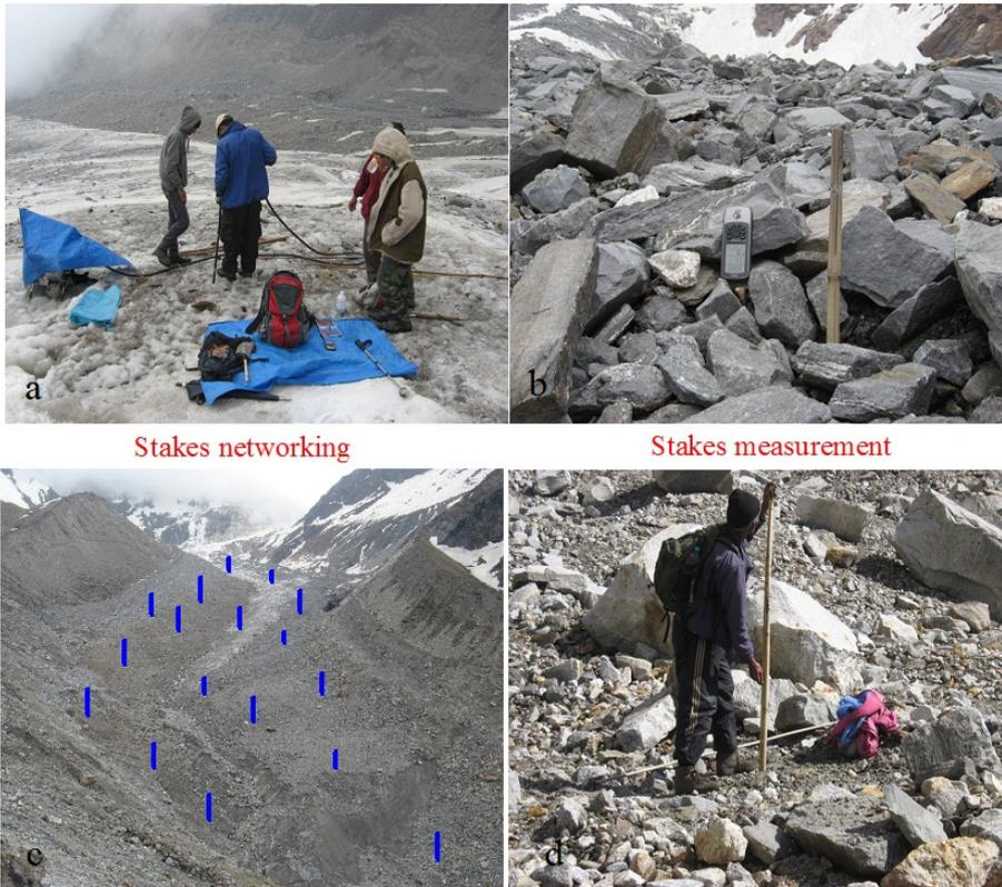
**Fig. 4.2:** Field work on the Dokriani Glacier for mass balance measurement (a) stream drill operation (b) stakes coordination (c) stakes networking and (d) stakes measurement.
