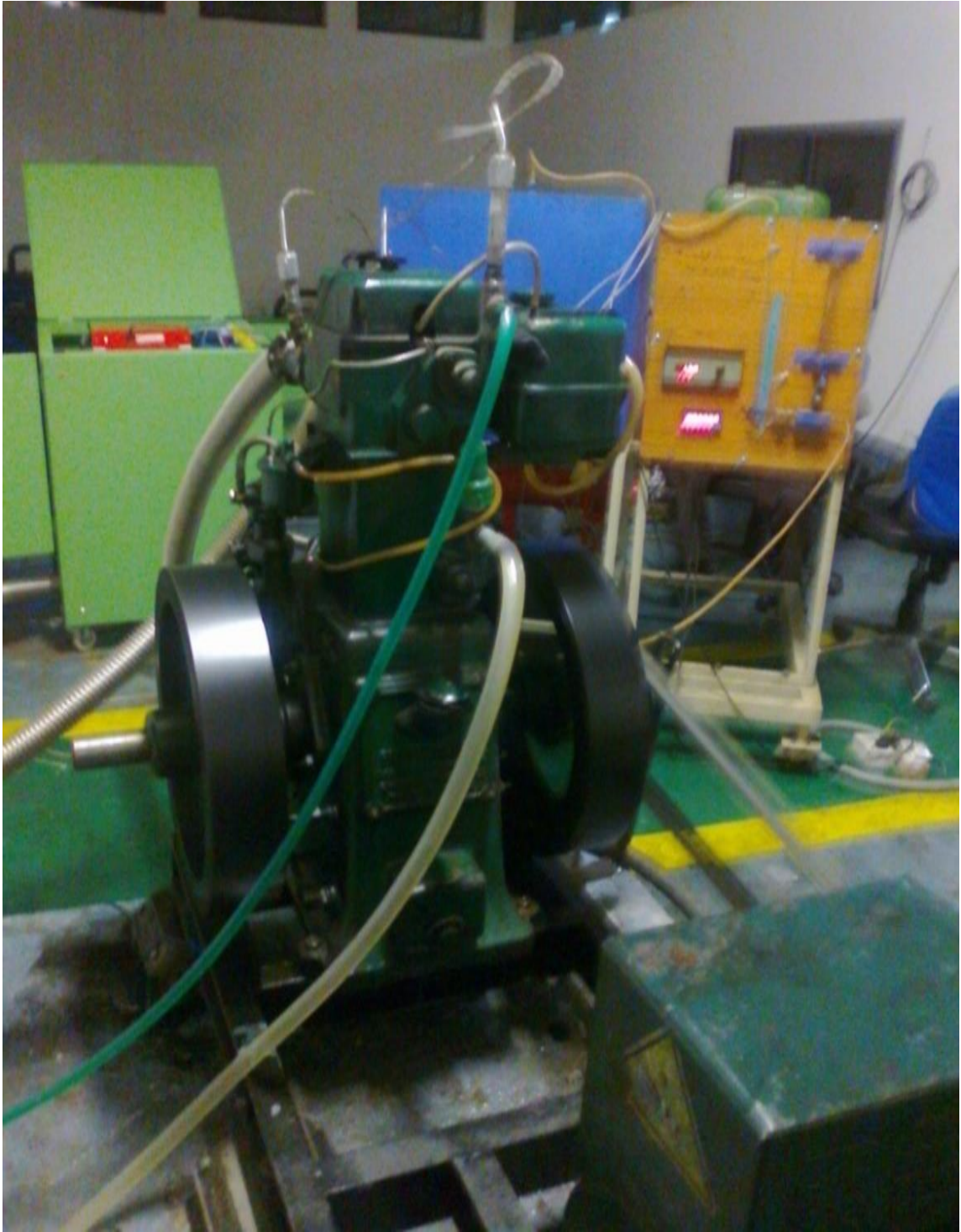
Figure 4.2: single cylinder IDI diesel engine.
