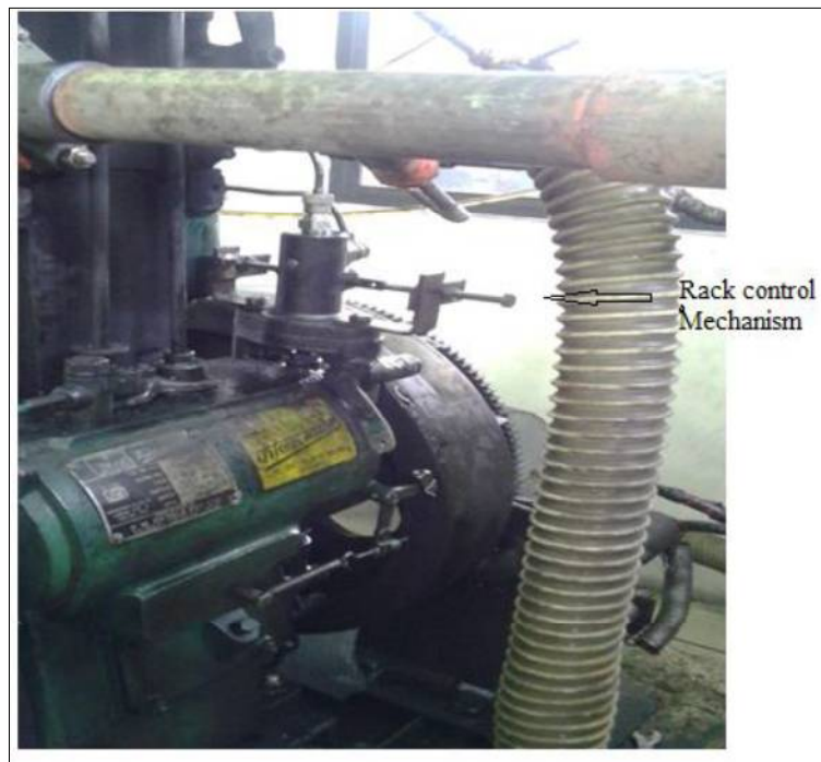
Figure 3.6 Rack control mechanism to run the engine at constant speed
