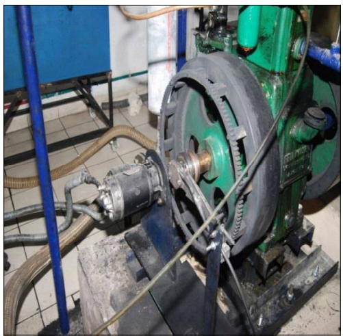
Figure AE.6 Development of self starting system
