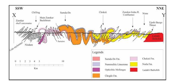
Figure 1.2 The structural cross-section along X-Y (shown in Fig 1.1), showing deformation of Indus basin sedimentary rocks (after Brookfield and Andrews-Speed, 1984). This small area (~35 km) has several north verging trusts and high angled reverse faults; Zanskar Back Thrust, Choksti thrust, and Upshi-Bazgo thrust.
