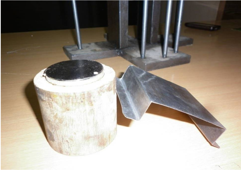
Figure 4.21: Fixed magnet and wooden cylinder with gate
