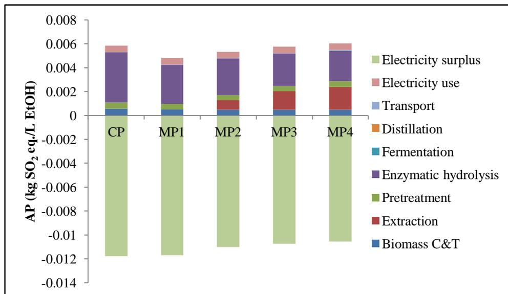
**Figure 6.5 AP of conventional and improved pretreatment method for ethanol production**
