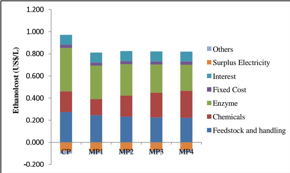
**Figure 6.8 Life cycle costing of the ethanol produced in different pretreatment scenarios**
