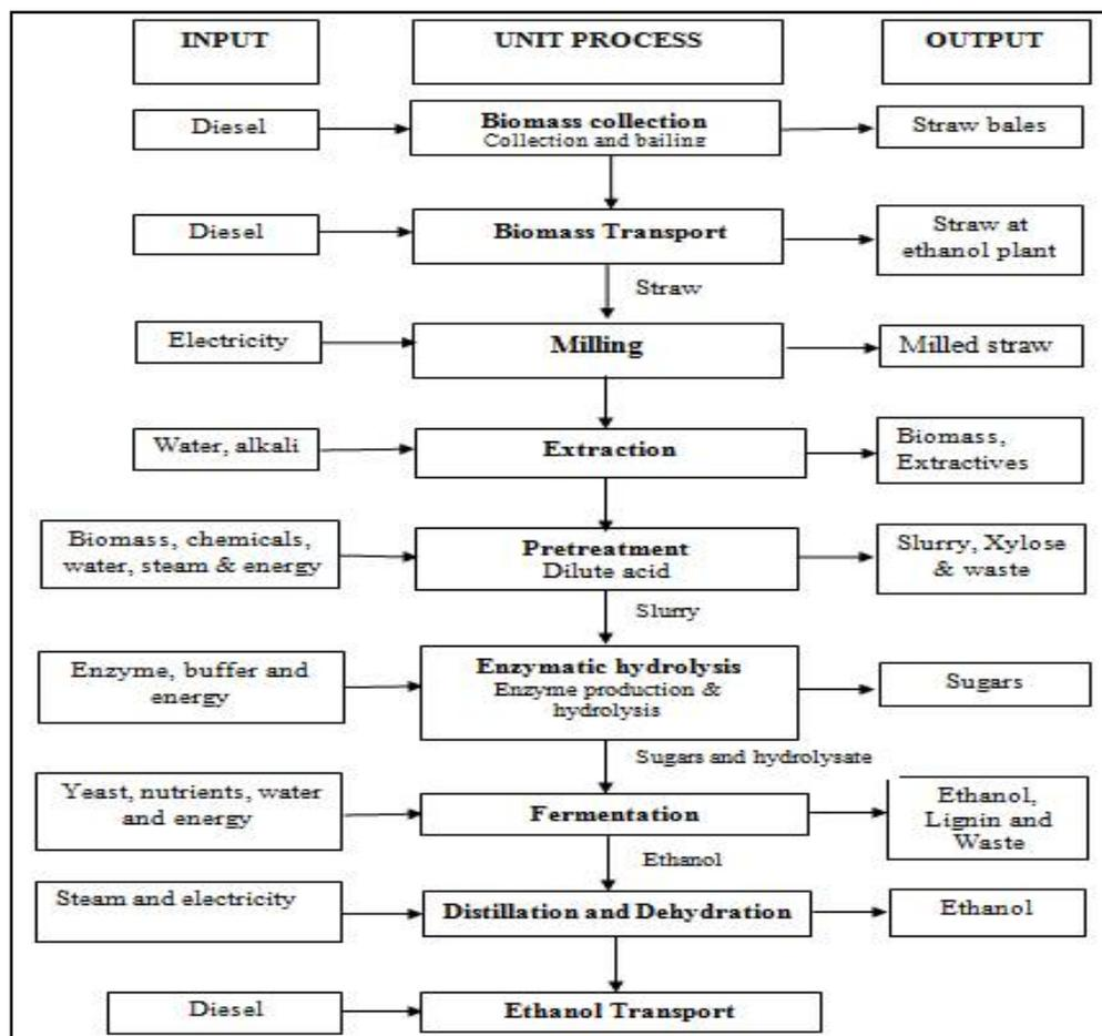
**Figure 6.2 System boundary of ethanol production**
