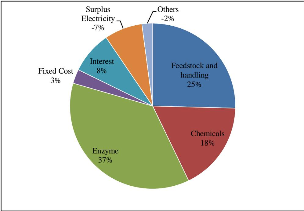
**Figure 6.7 Conversion cost breakdown in an ethanol plant**
