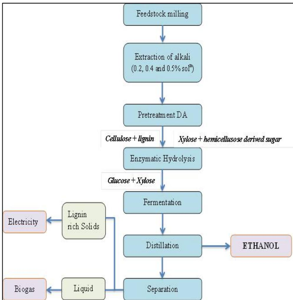
**Figure 6.1 IOCL advanced pretreatment technology for ethanol production**
