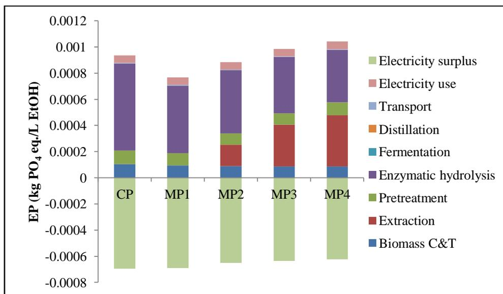
**Figure 6.4 EP of conventional and improved pretreatment method for ethanol production**
