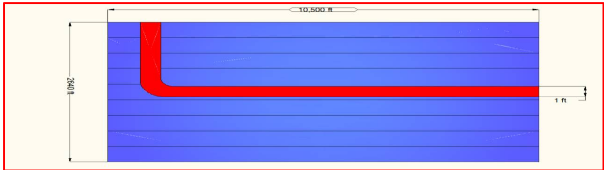
Figure 3.5: Schematic Representation of Wellbore in the 5 th Layer from Top.
