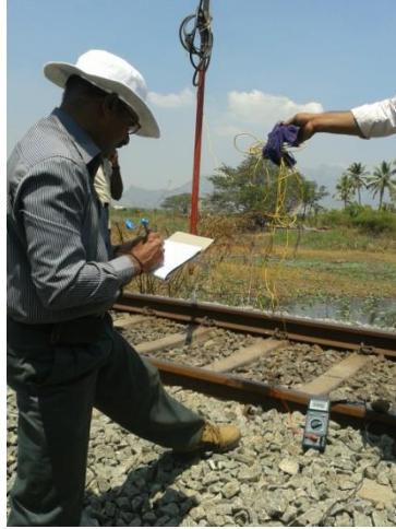
Fig.3.4 Validation test conducted on an actual 25 kV electric traction system.
