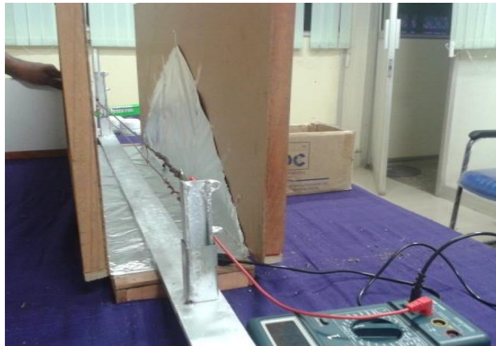
Fig.4.3 Experiment on model of OHE at laboratory at different angles and different base widths.
