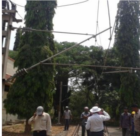
Fig.3.2 Experiment conducted on a 50 m long prototype of conventional OHE
