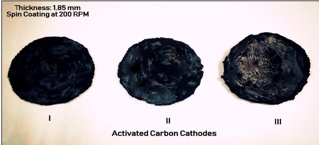
**Figure 4.15:** AC+CB+PVDF cathodes fabricated via single step phase inversion process.
