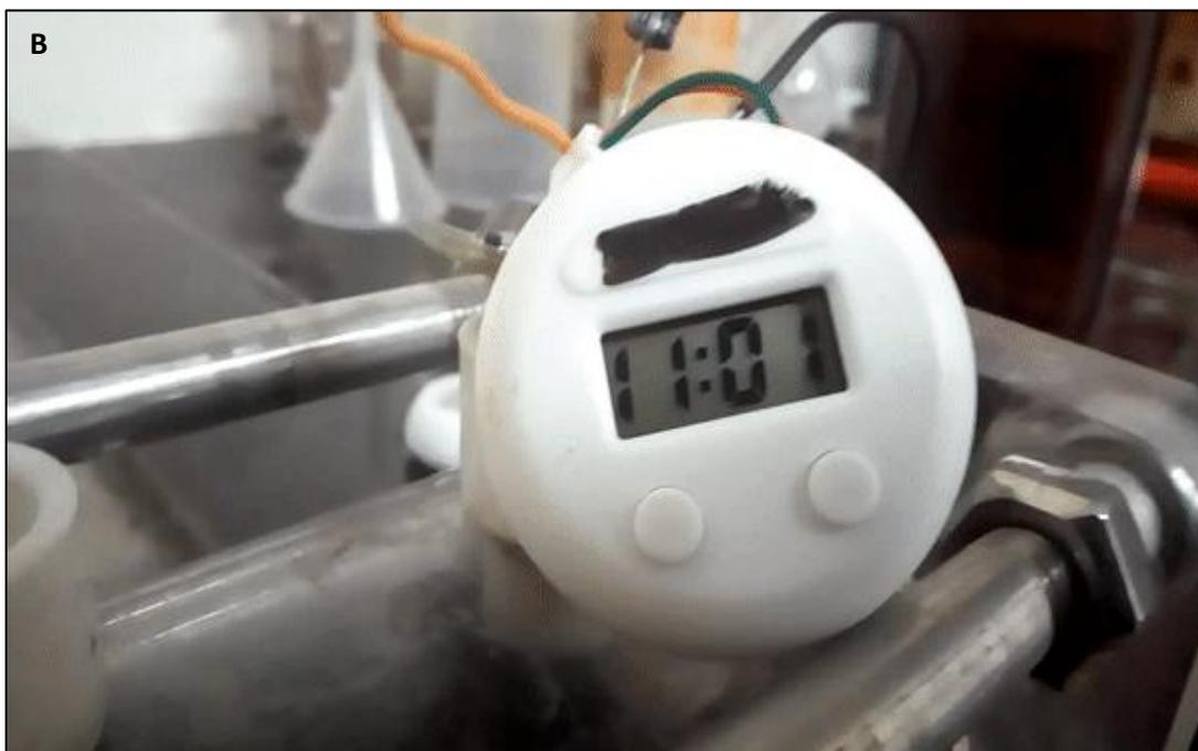
**Figure S4-2:** Portable electronics powered using wastewater by connecting (A) LED (B) Digital watch to the anode and the cathode wiring.
