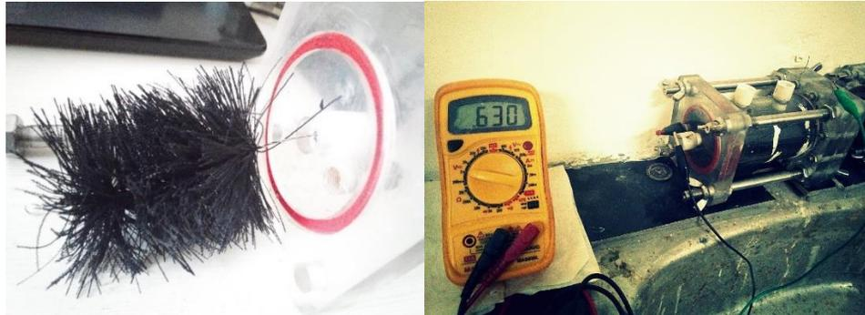
**Figure 4.17:** Carbon yarn based brush attached to titanium wires shown at the right, Brush anode based membrane-less air cathode MFC in operation showing OCV close to the range of Pt-Catalyst system, here it is 0.63 V or 630 mV.
