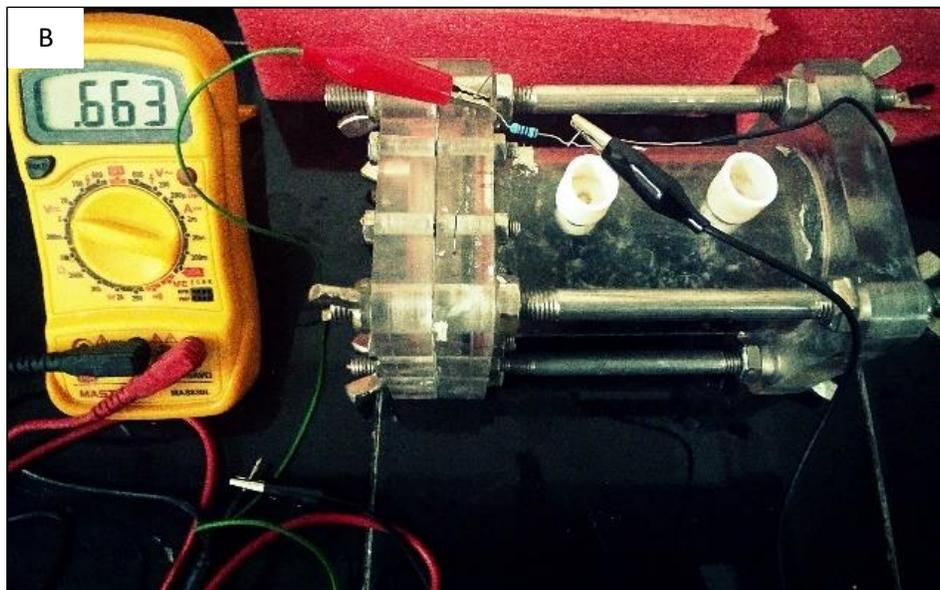
**Figure 4.22:** (A) Polarization curves for the AC-Cat MFC (B) System connected to a low external resistance, in this case achieved 0.663 V with a 500 ohms external resistor.
