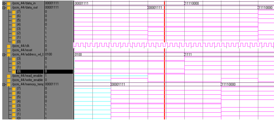
Fig. 6.7 Modelsim simulation of PCM array (4 x 4)
