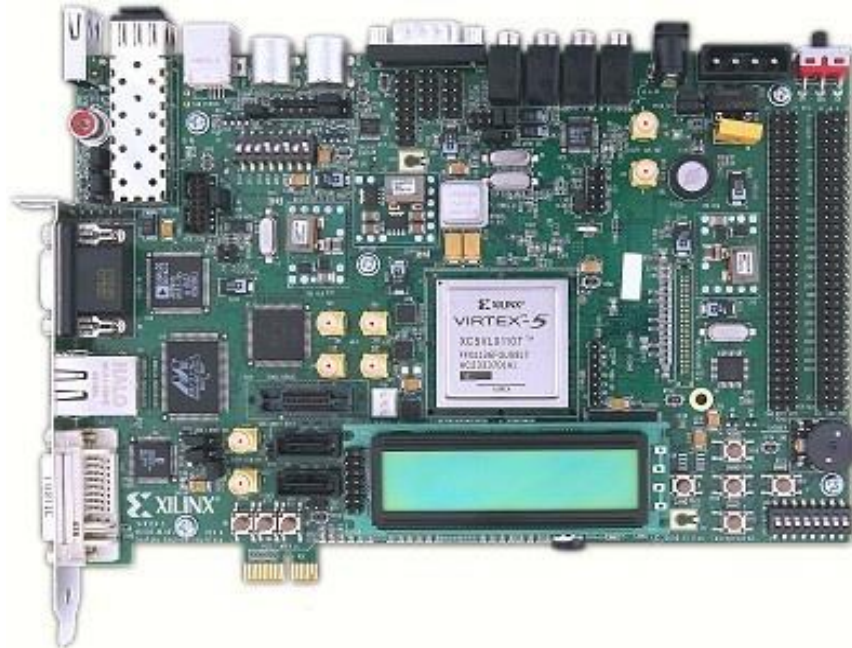
Fig. 6.19 Functional view of FPGA Virtex – 5 FPGA
