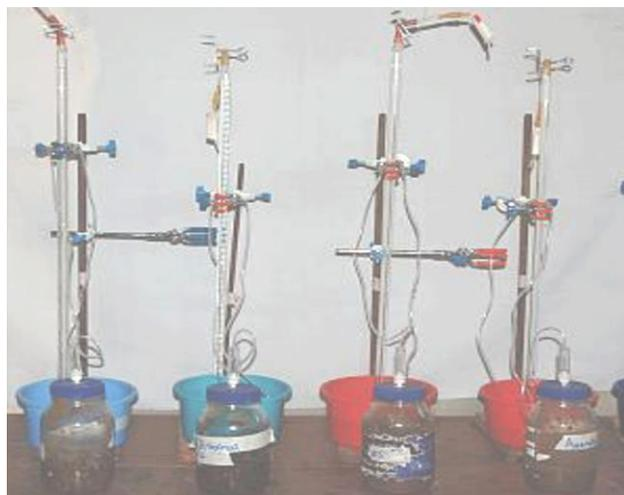
**Fig. 4.2 Batch stirred tank reactor with water displacement**
