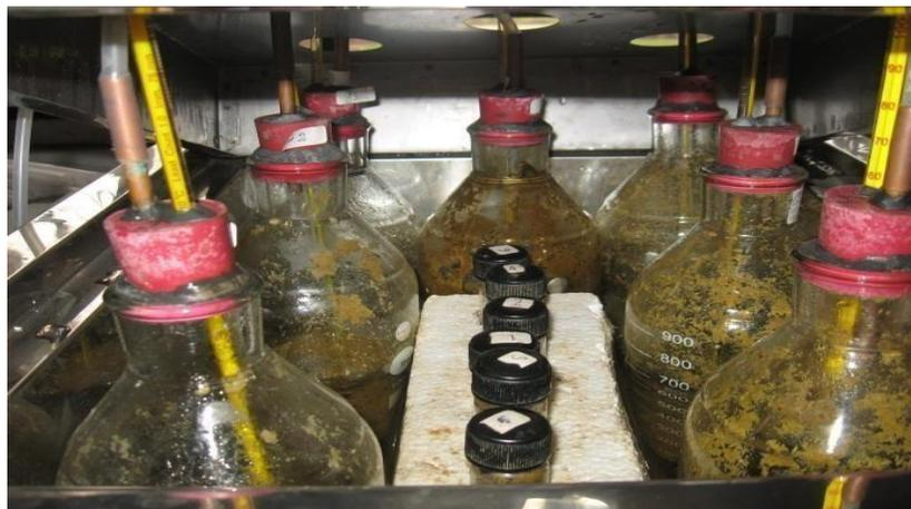
**Fig. IV.2** Small scale digesters inside water bath kept for fermentation
