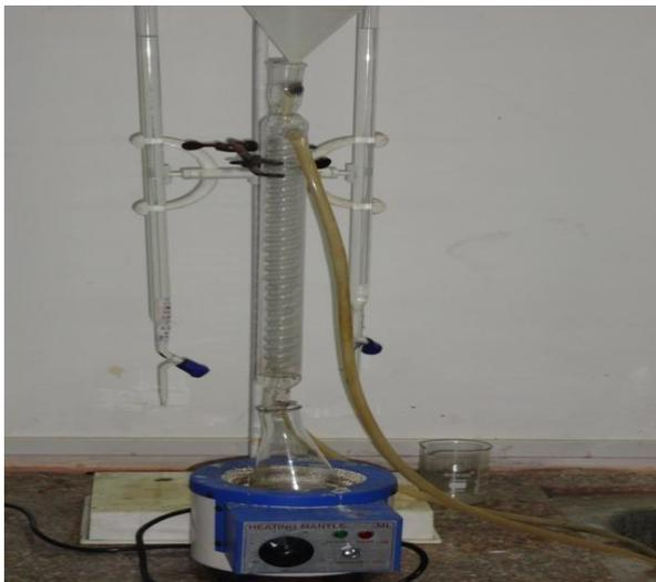
**Fig. IV.6 Set-up for COD with heating mantle**
