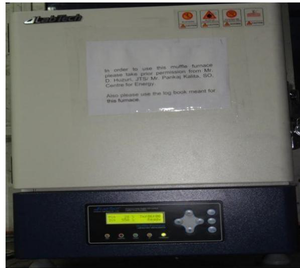
**Fig. IV.5 Muffle Furnace**
