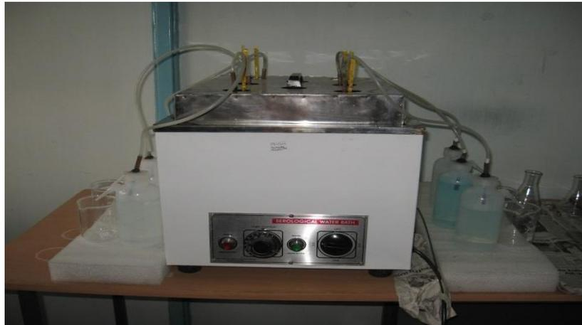
**Fig. IV.1** Waterbath where smallscale digesters were kept for fermentation under constant temperature condition
