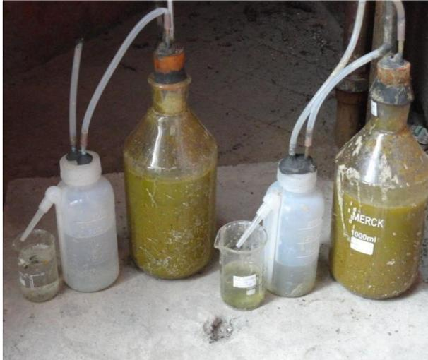
**Fig. IV.8 Laboratory scale digesters**
