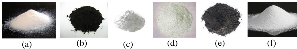
Fig. 1.7: Images of different nanoparticles included in this study. (a) \text{SiO}_2 NP (b) \text{CuO} NP (c) \text{Al}_2\text{O}_3 NP (d) \text{ZrO}_2 NP (e) GO NS (f) \text{ZnO} NP
