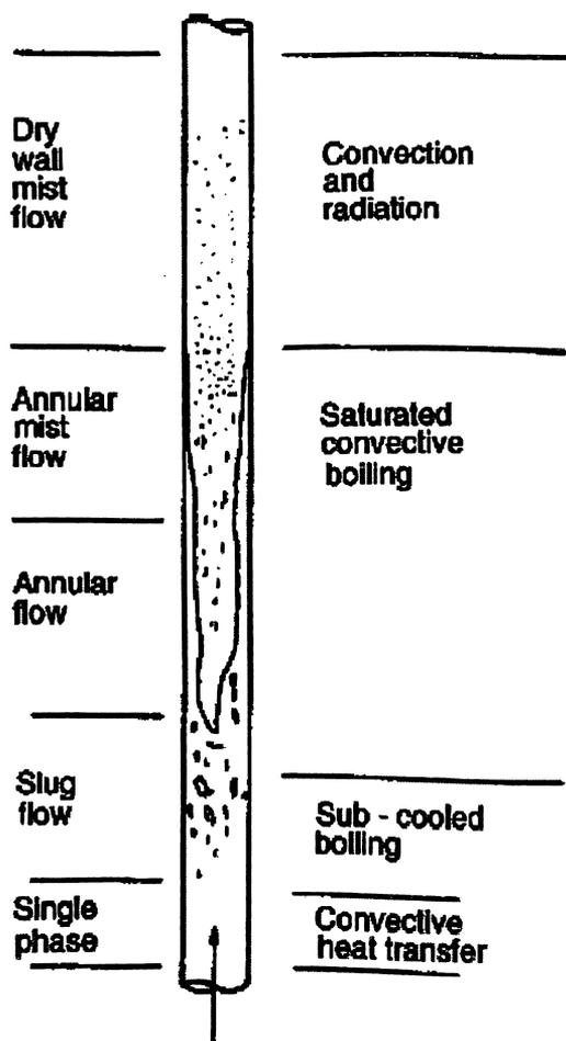
3. Saturated boiling region: in this region bulk boiling of the liquid is occurring in a manner similar to nucleate pool boiling. The volume of vapour is increasing and various flow patterns can form (see Volume 2, Chapter 14). In a long tube, the flow pattern will eventually become annular: where the liquid phase is spread over the tube wall and the vapour flows up the central core.
