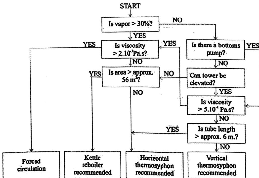
Fig. Basic reboiler design selection algorithm
