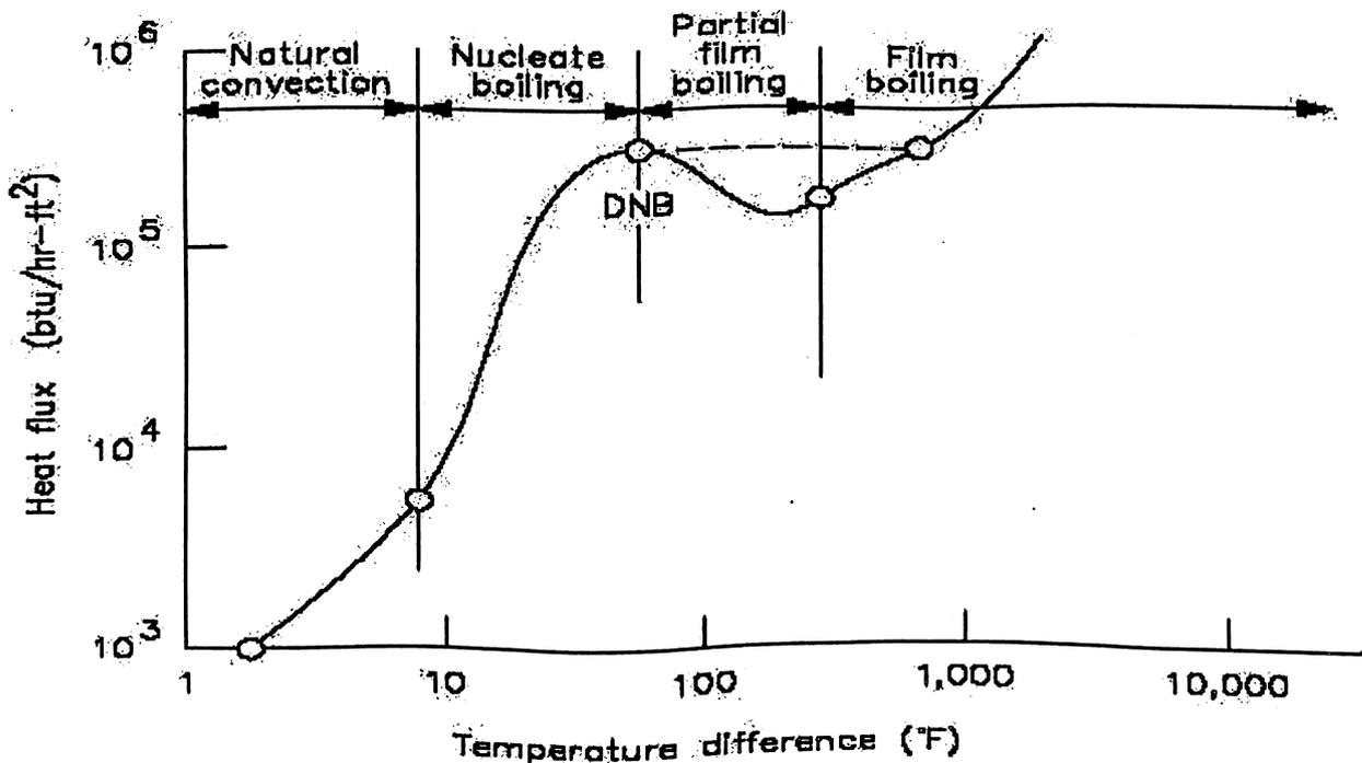
The maximum heat flux achievable with nucleate boiling is known as the critical heat flux. In a system where the surface temperature is not self-limiting, such as a nuclear reactor fuel element, operation above the critical flux will result in a rapid increase in the surface temperature, and in the extreme situation the surface will melt. This phenomenon is known as "burn-out". The heating media used for process plant are
