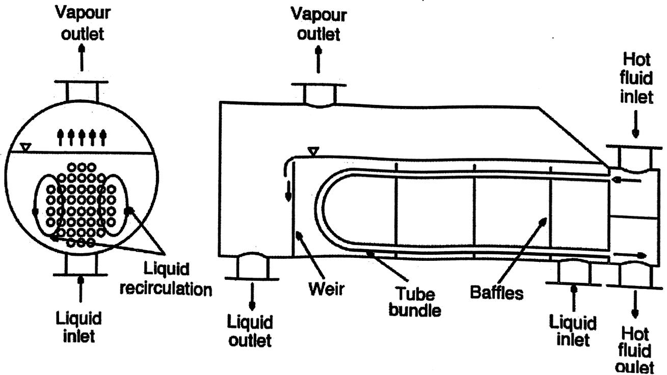
(Fig1: Schematic view of kettle type reboiler)
