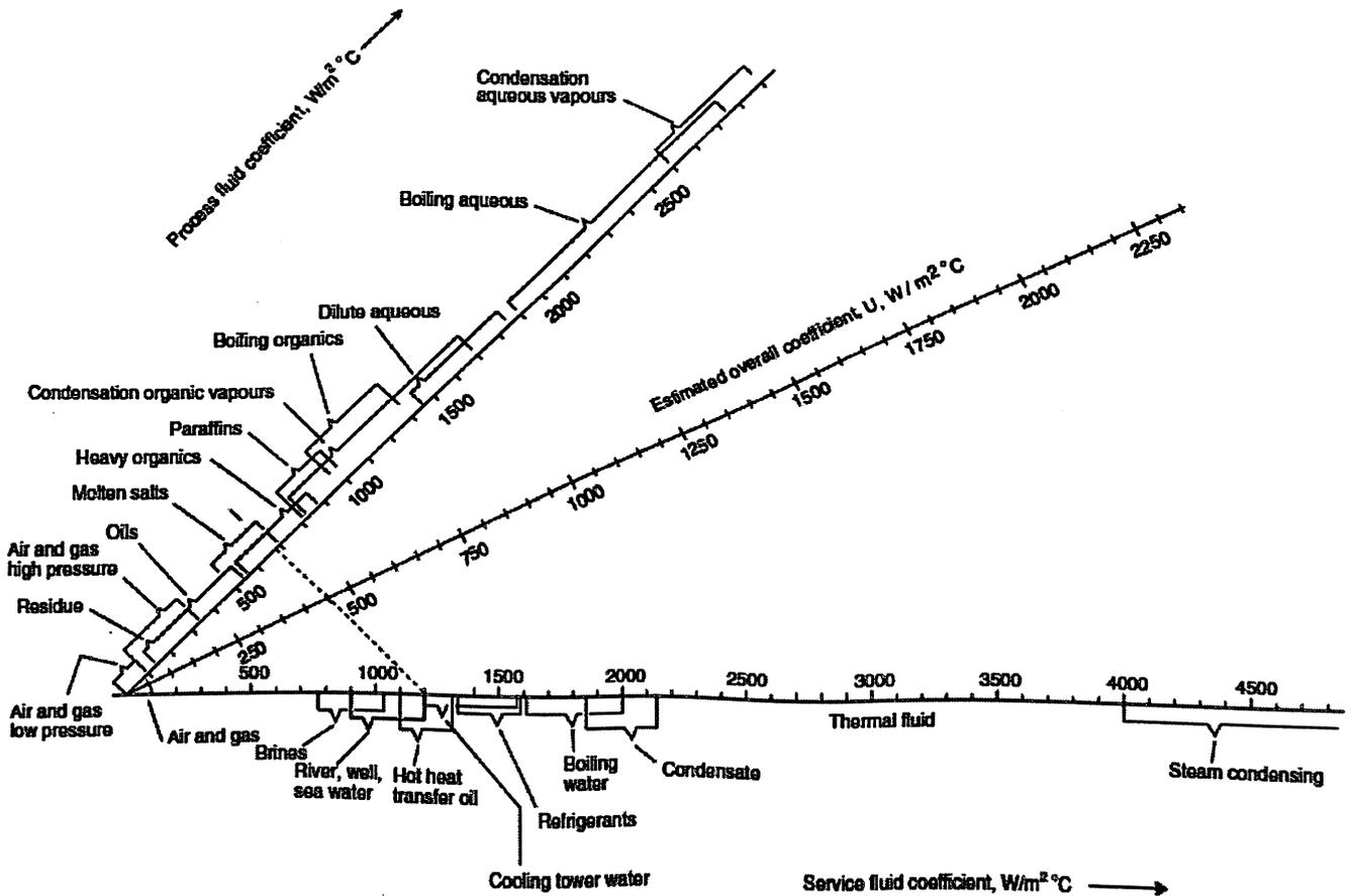
Overall coefficients (join process side duty to service side and read U from centre scale)
