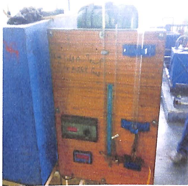
Figure 3.2:Fuel inlet and controller
