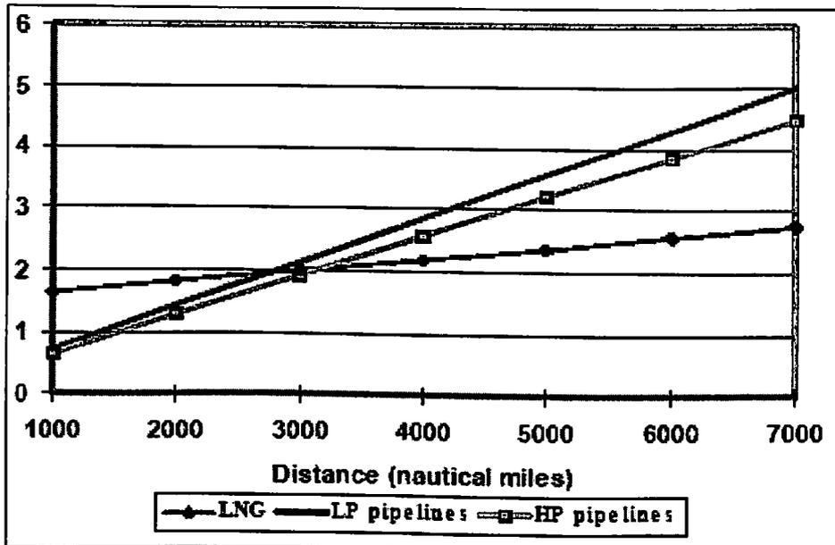
Figure 25 Pipes /LNG competition for  $10 \times 10^9 \text{ m}^3 / \text{year}$  capacity, in USD / MM BTU
