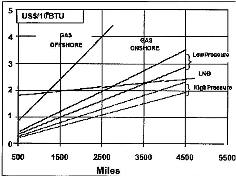
Figure 24 Pipes /LNG competition for  $30 \times 10^9 \text{ m}^3 / \text{year}$  capacity. Source ENI.
