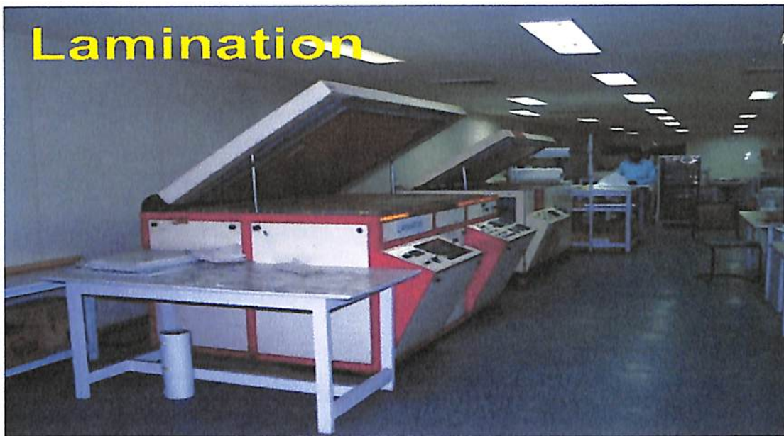
Fig.5: lamination of the solar module
