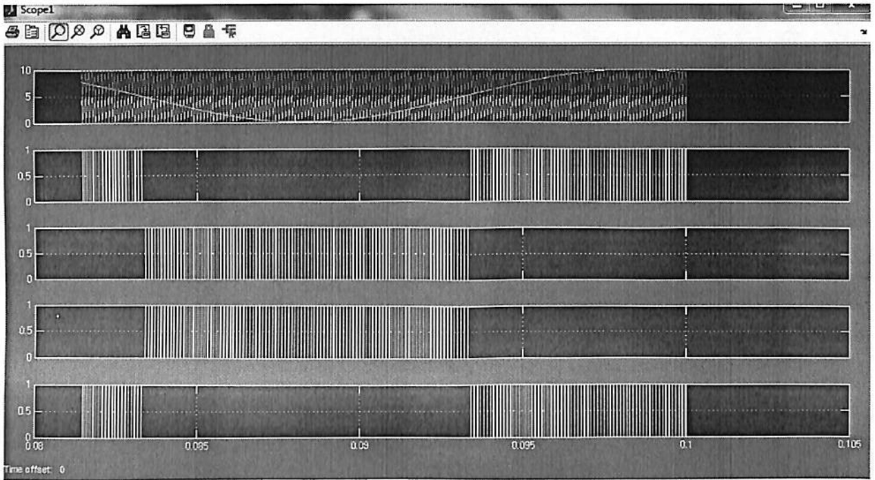
Fig.-61 Input Signal with 120 degrees phase delay
