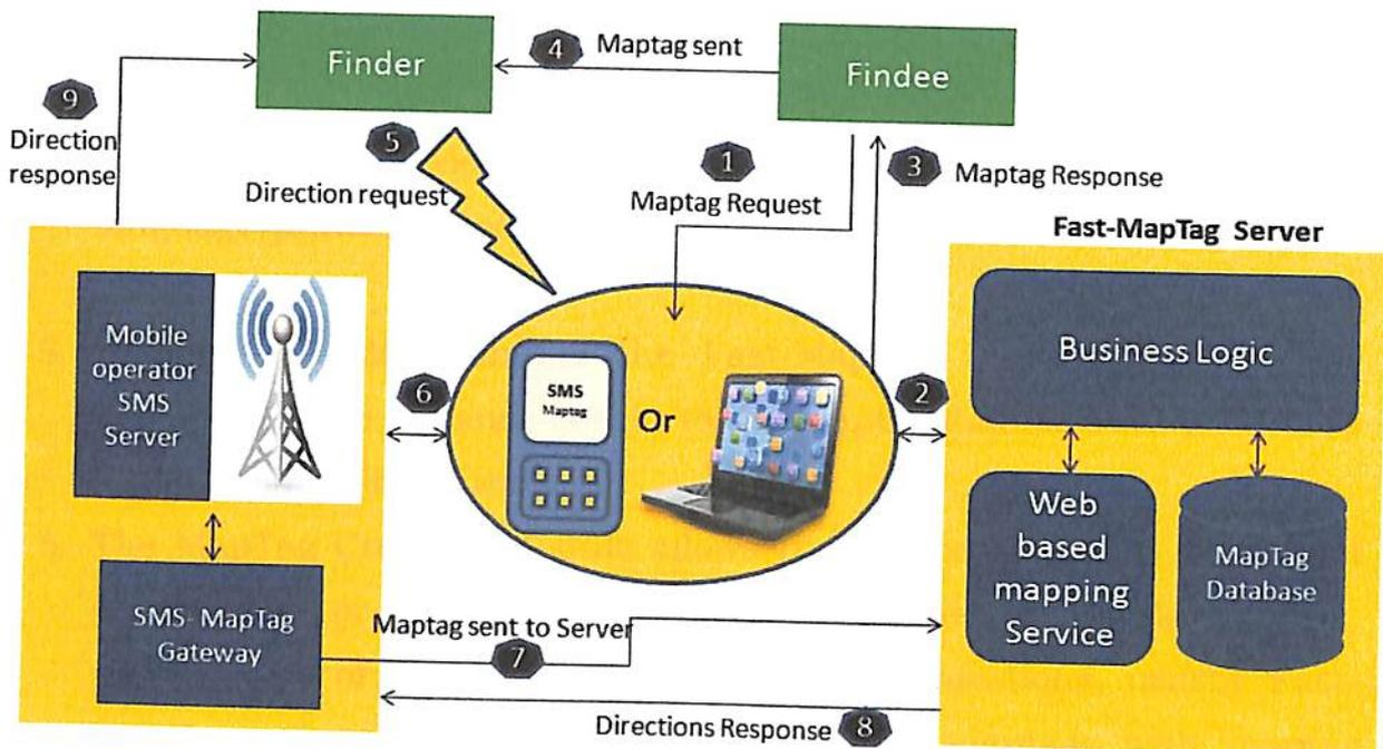
Fig.5.1 Fast map tag system flow
