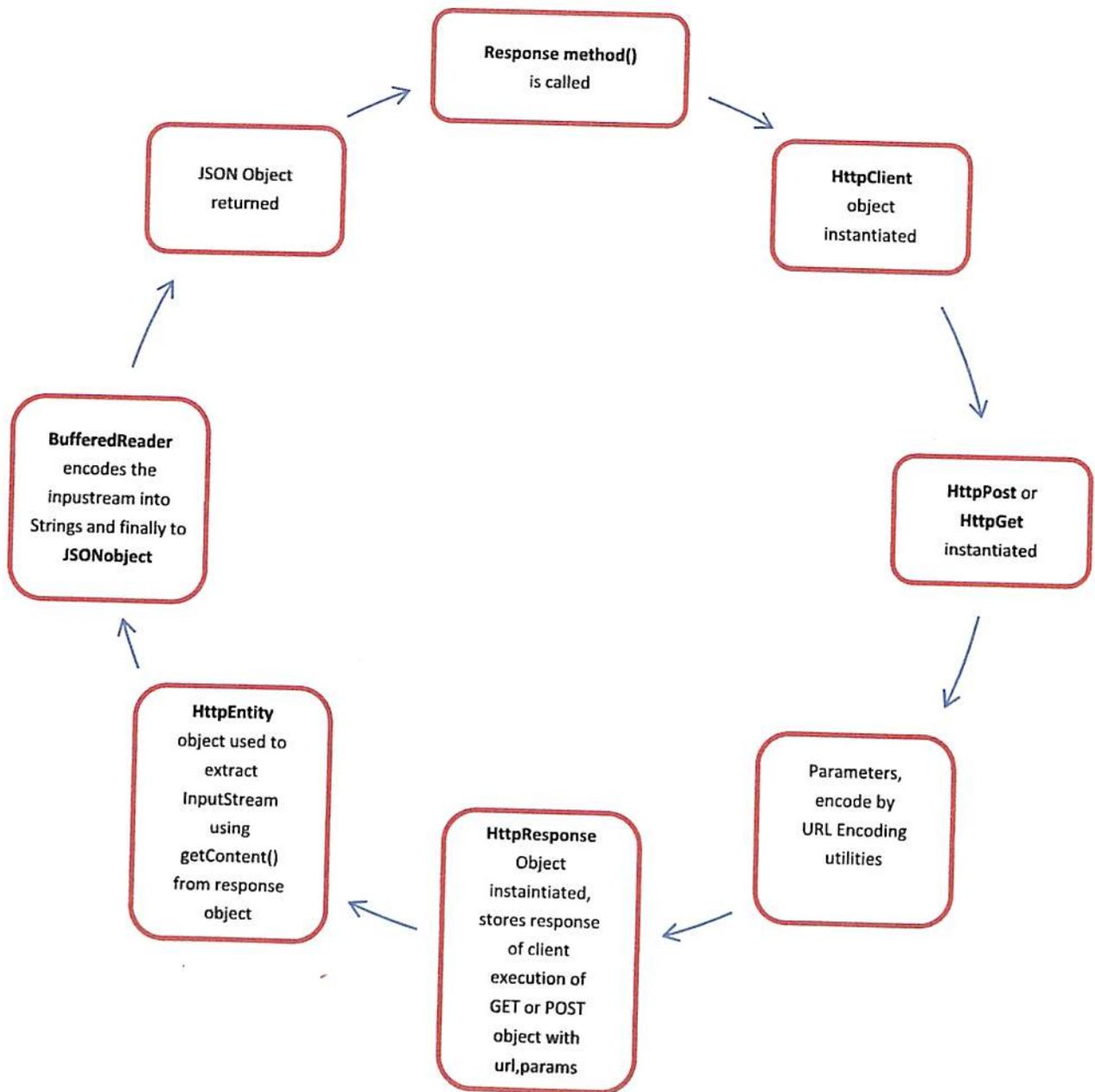
Fig6.2 Response method() execution cycle in Android
