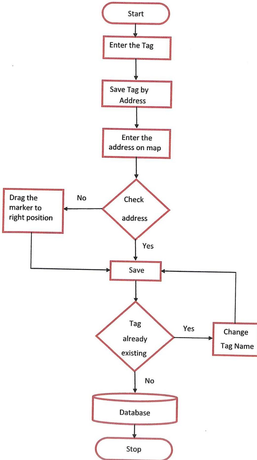
Fig 6.4 Flow chart of creating tag and save with address
