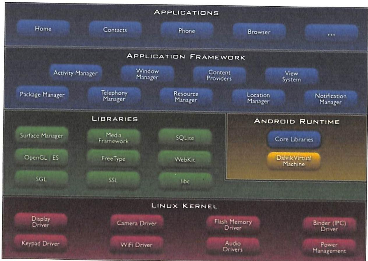
Fig. 3.1 Android Architecture [Courtesy Source: <http://developer.android.com/guide/basics/what-is-android.html>]
