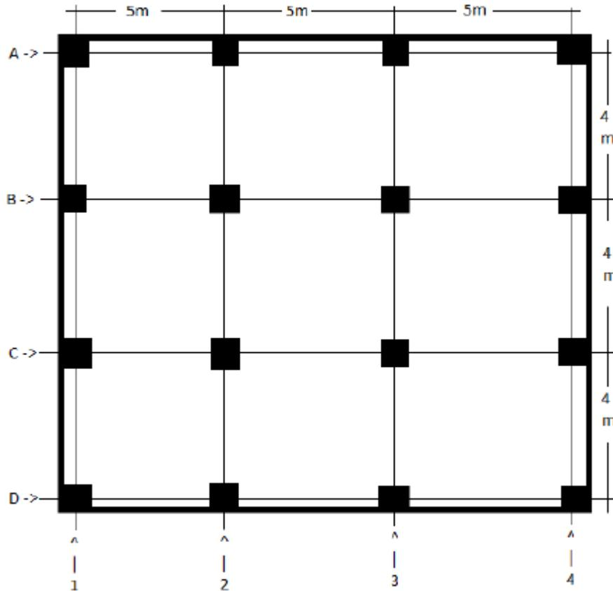
The columns D1, D2, D3, D4 terminate at single storey. The columns A1, A2, B1, B2, C1, C2 terminate at double storey. Rest of columns terminate at eight storeys. Assume suitable projections at the base. Assume column size as 400x400mm and density of soil as  $17 \text{ KN/m}^3$  and M40 grade concrete.
