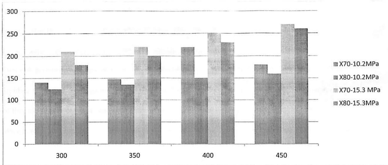
Figure 3: Force to puncture with tiger tooth
