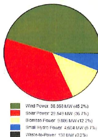
Figure 3.4: Installed grid interactive renewable power capacity in India as of 30 June 2019 (excluding large hydro)
