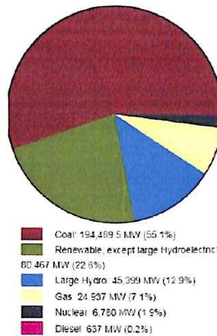
Figure 3.3: Installed grid power capacity from all sources in India as of 30 June 2019
