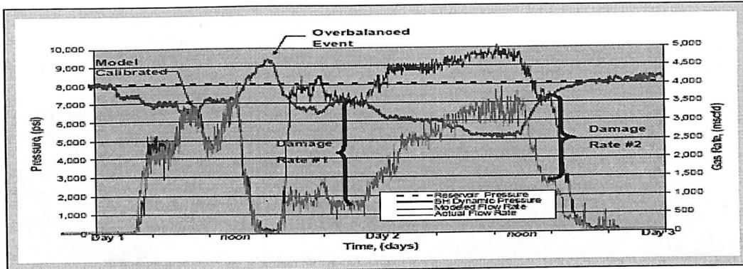
Figure 2: Simulated Underbalanced Job Chart with Overbalanced Event (composite of field cases)
