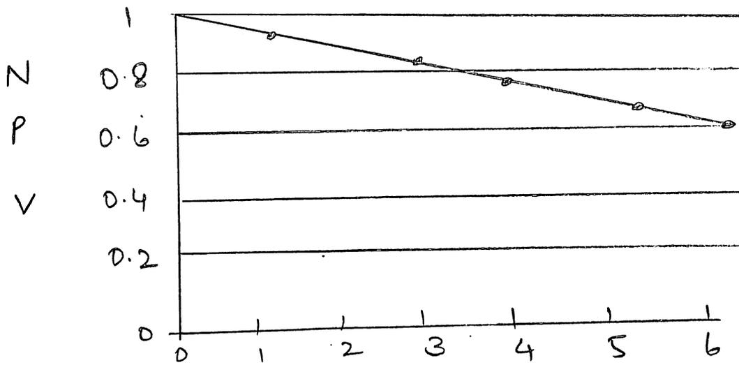
The increased production is based on a lower abandonment pressure before the well reaches its economic production limit. The following figure is an example of the difference in abandonment pressures.
