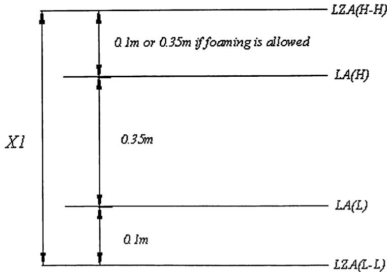
The values given here are for the minimum distance between the levels the final values are found after checking the control time for each level.
