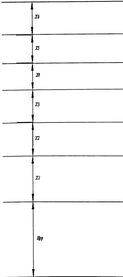
X6 is the distance between top of demisting internals and TTL  $X6 \approx 0.15D \geq 0.15m$
