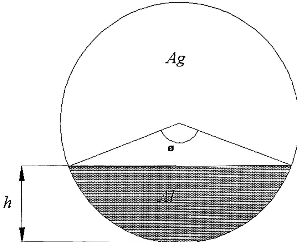
The positions of the liquid and gas phases have been indicated and have a cross-section area  $A_g, A_l$ .
