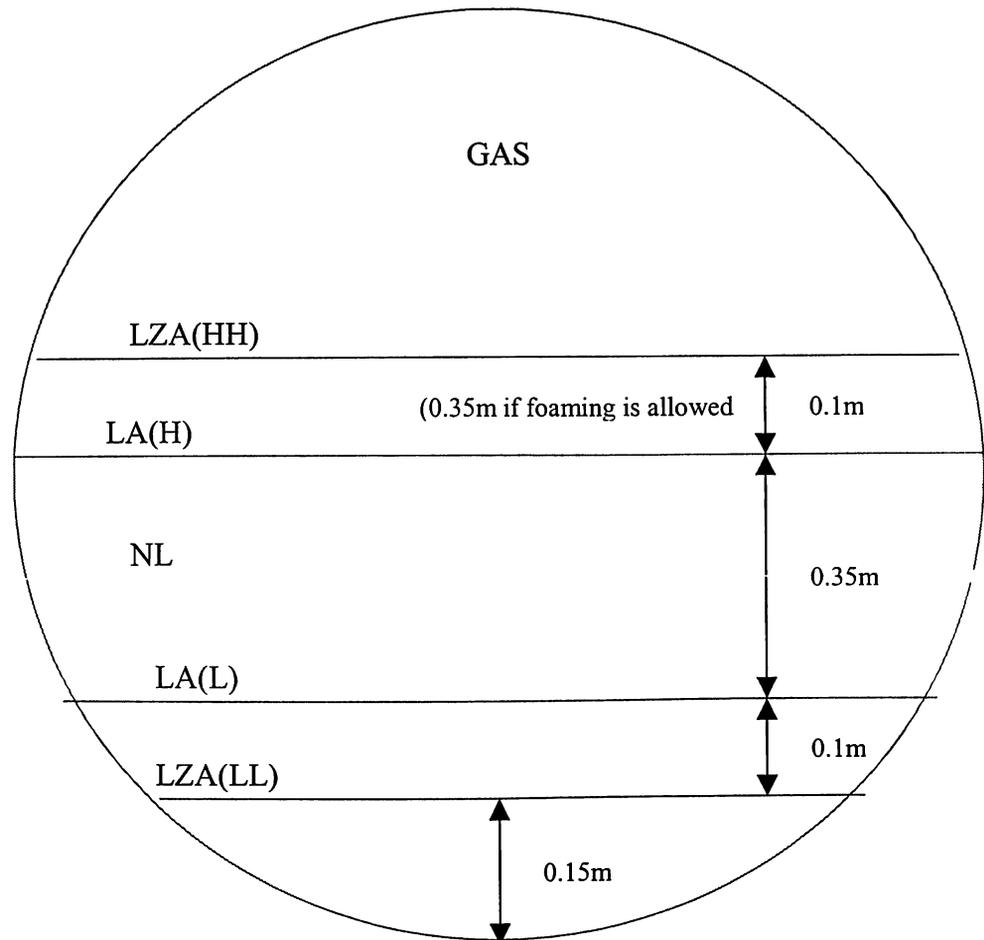
1. LZA (LL)-Low level trip; is 0.15 m above the bottom of the vessel i.e 0.15 from BTL (Bottom Tangent line) and 0.15m from bottom of the Horizontal Separator
