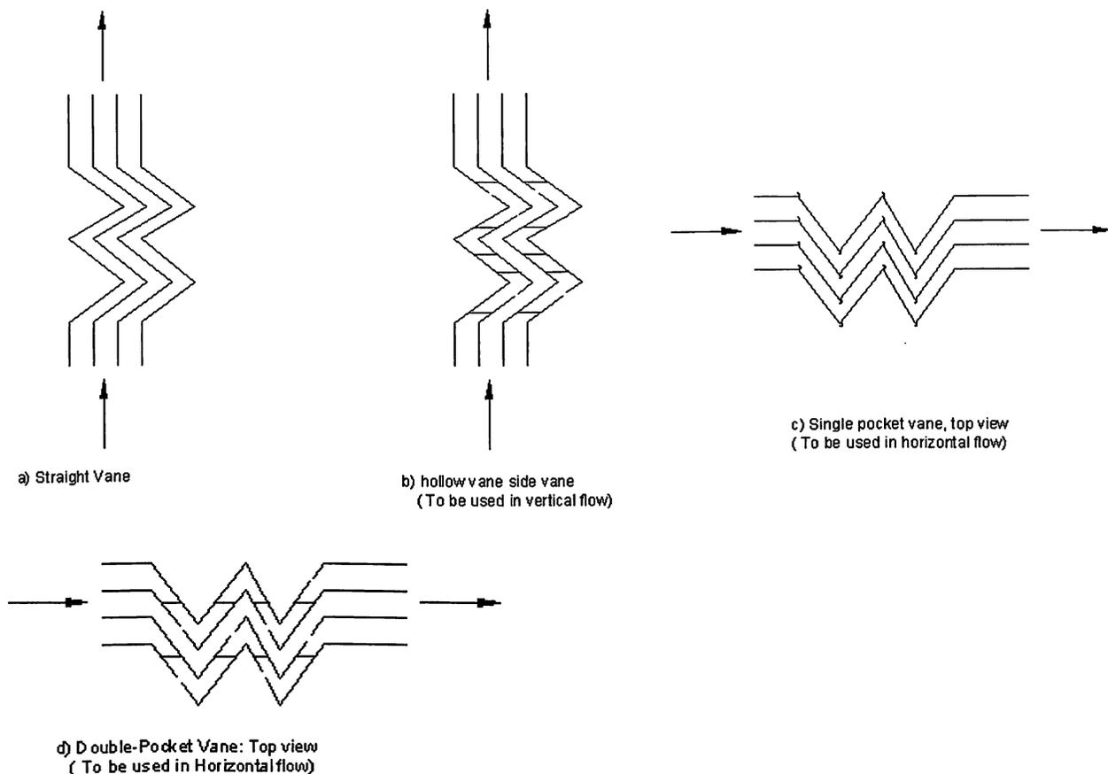
Of the three types the straight vane has the lowest liquid separation efficiency. The double-Pocket vane type has the highest sensitivity to fouling but its efficiency above  $\lambda_{\text{max}}$  (Where liquid re-entrainment starts) Deteriorates to a lesser degree than with the other types because the separated liquid is better shielded from the gas flow.
