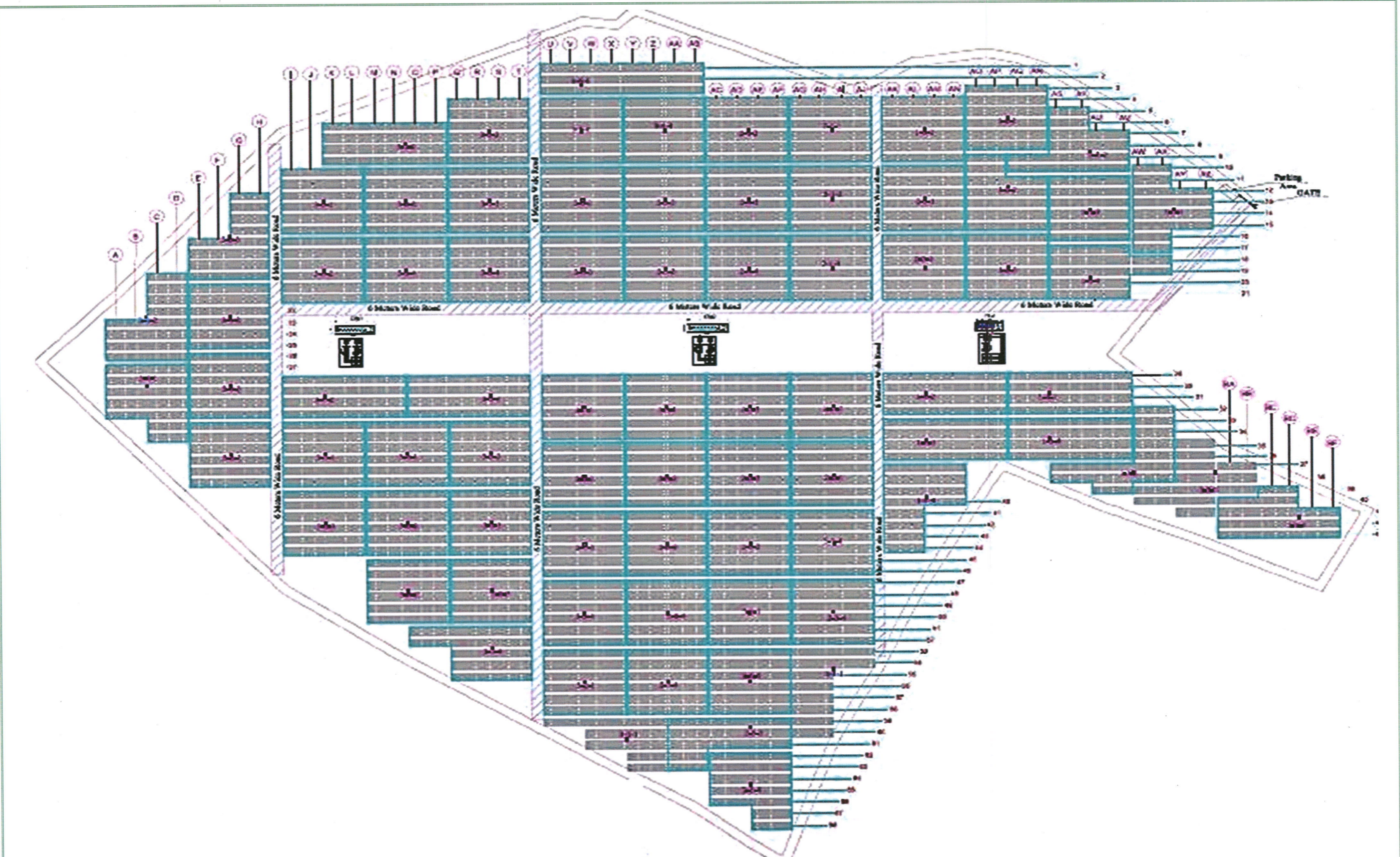
Figure 4.6: 10MW Solar power plant array layout
