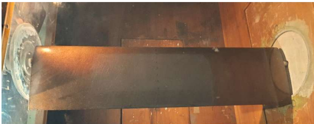
Figure 3.26 a) SRM IST – KTR low subsonic wind tunnel with pressure scanner setup. b) Infinite wing model inside the test section.
