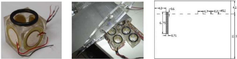
Figure 2.5: The synthetic jet actuator arrays on wing (Tang et al. 2014).
