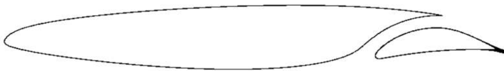
Figure 2.43: The slotted, Natural Laminar flow S103 airfoil (Somers, 2012).
