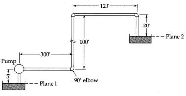
Fig. 1. Pipeline flow with friction losses because of fittings. Planes 1 and 2 are just under the surface of the liquid.
