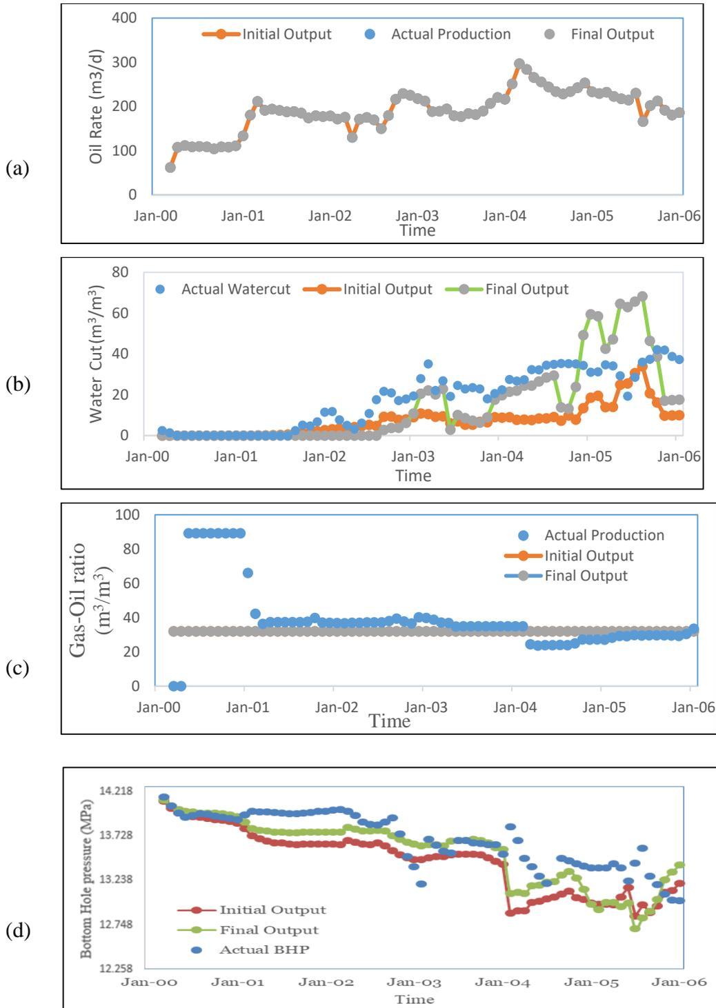
Figure 5.5 Case (a) - Comparison of simulator output of best final ensemble (after optimization) with observed field values and best initial ensemble (before optimization) for (a) Oil rate (b) Water cut (c) GOR and (d) BHP
