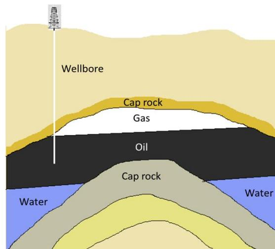
Figure 1.1: Schematic of a Hydrocarbon reservoir
