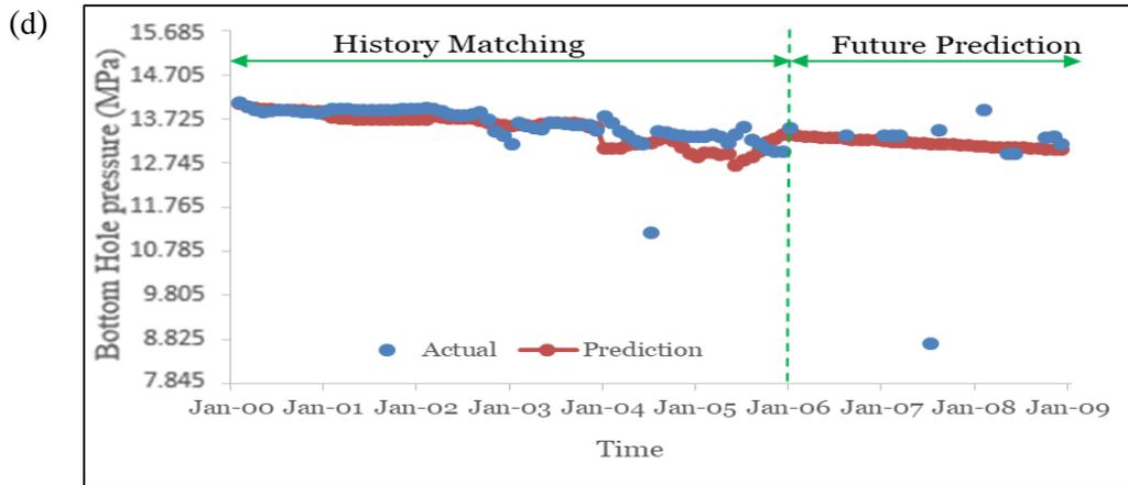
Figure 5.8: Comparison of predictions from the model with the field observations (a) Oil rate (b) GOR (c) Water cut and (d) BHP
