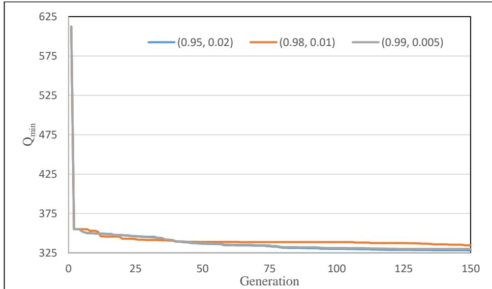
Figure 5.6: Variation of objective function ‘ $Q_{\min}$ ’ with generations for  $(P_c, P_m) = (0.95, 0.02), (0.98, 0.01)$  and  $(0.99, 0.005)$  for case (b)
