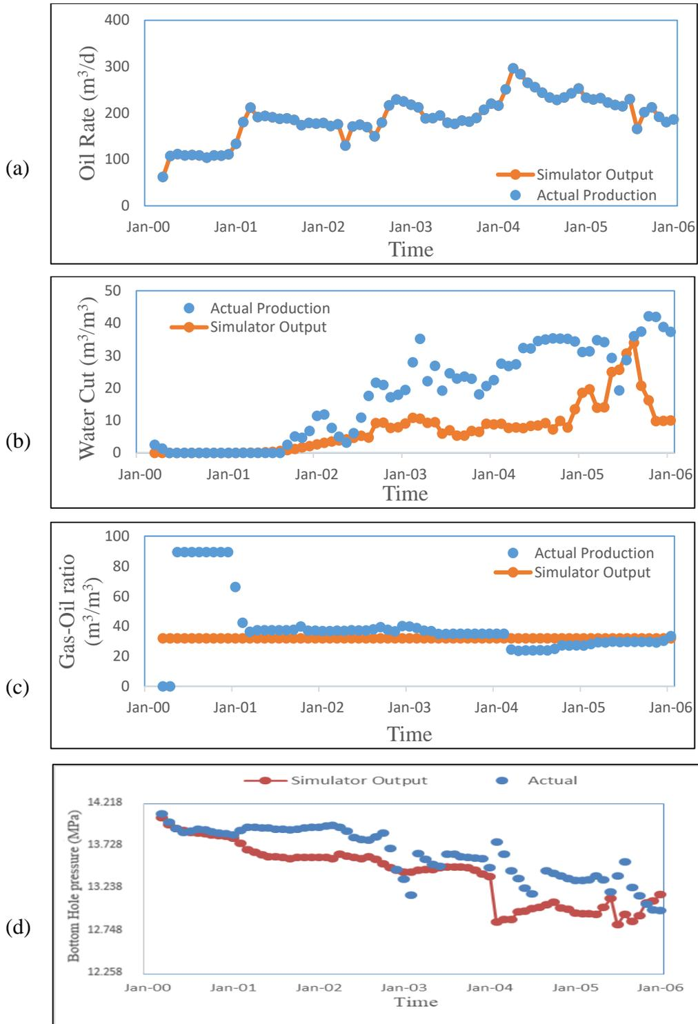
Figure 5.3 Case (a) - Comparison of simulator output of best initial ensemble (before optimization) with observed field values for (a) Oil rate (b) Water cut (c) GOR and (d) BHP
