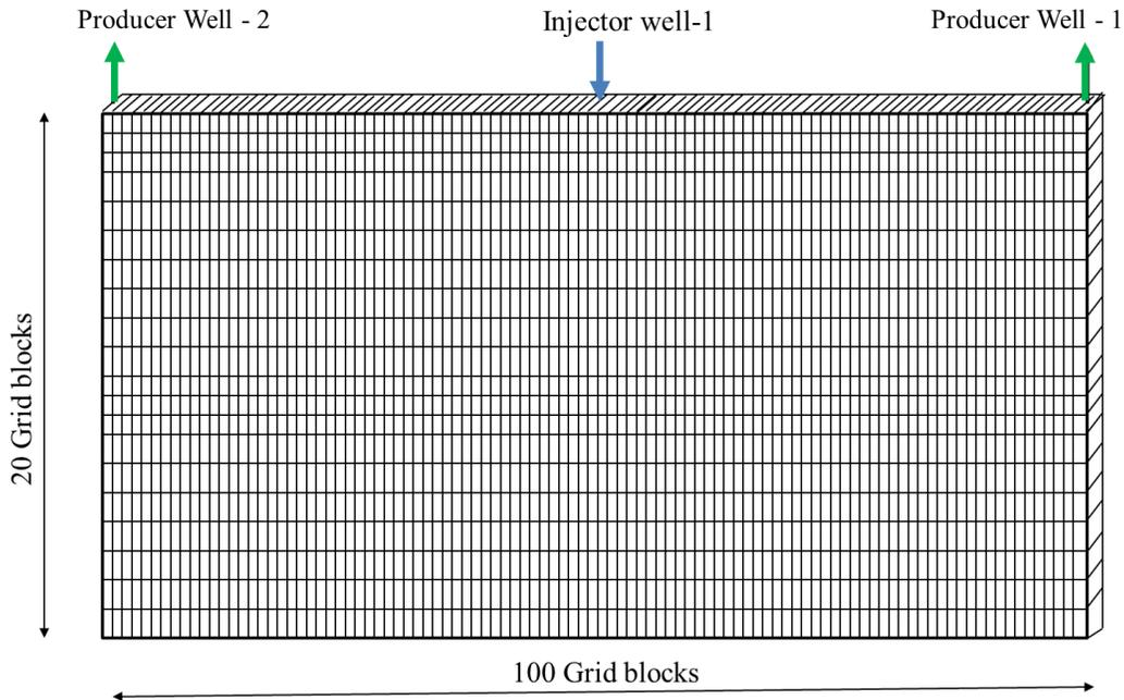
Figure 4.3: Schematic of synthetic reservoir
