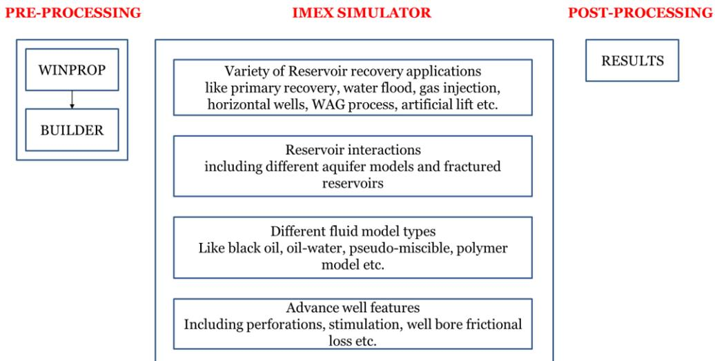
Figure 3.2: Schematic of CMG<sup>®</sup> IMEX<sup>™</sup> Simulator
