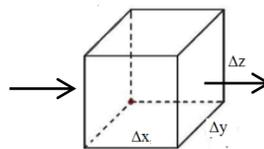
Figure 3.1: Element of a reservoir with dimensions Δx, Δy and Δz
