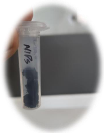
Figure 3.8. The dried solid polyaniline after the oxidative polymerization of aniline
