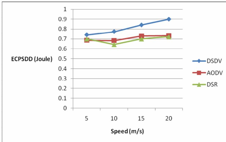
**Fig. 4.11 (b): Energy Consumption per Successful Data Delivery Vs Speed**
