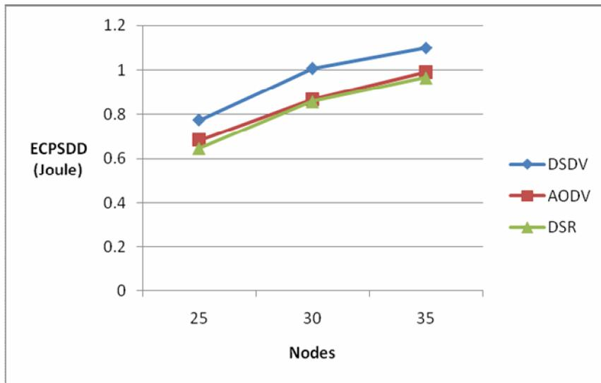
**Fig. 4.11 (a): Energy Consumption per Successful Data Delivery Vs Nodes**
