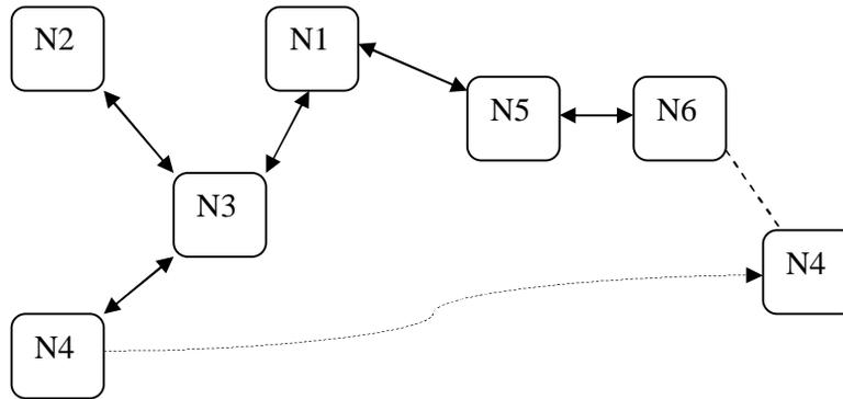
**Fig 3.2: Example Network for DSDV**
