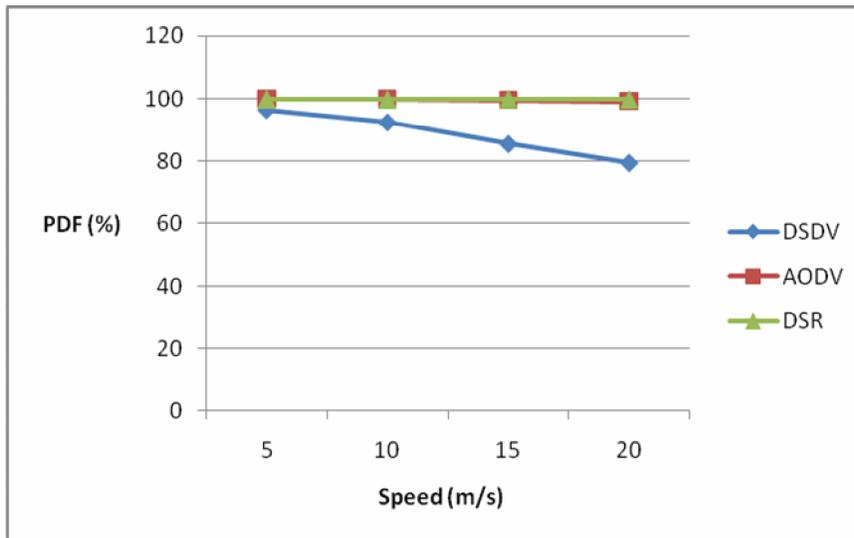
**Fig. 4.10 (b): Packet Delivery Fraction Vs Speed**
