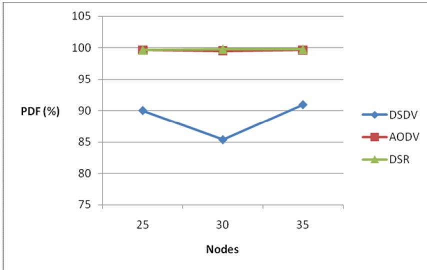
**Fig. 4.10 (a): Packet Delivery Fraction Vs Nodes**
