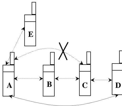
**Fig. 3.1: An ad hoc wireless network**
